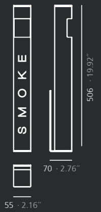
FUMPA Wall hanged ashtray column Capacity: 0.7 liters Columna cenicero a pared Capacidad: 0.7 litros
