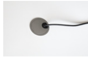
Grommet cover round 80mm for tabletop: Manufactured in Zamak alloy, finished in matt chrome with a black rubber cable grommet. The drill hole in the cover to facilitate insertion must be done by the customer.
