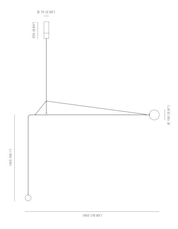
66.35~50W / 12V frosted halogen for ø150mm sphere 760~lm / 2700K
