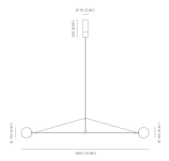
$66.35\ 50W\ /\ 12V$  frosted halogen for ø150mm sphere  $760\ lm\ /\ 2700K$
