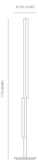
Bulb specifications 240V S14s opal LED tube Radium Raledina 16,5W / 1000mm Ø 29mm 1000lm / 2700K
