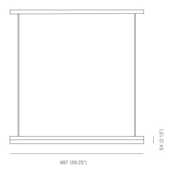
Bulb specifications 240V S14s opal LED tube Radium Raledina 16,5W / 1000mm Ø 29mm 1000lm / 2700K
