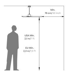
Allow a minimum clearance of 2,1 m (7 ft) for USA and 2,3 m (7,5 ft) for Europe from the floor to the blades and 30 inches (76 cm) from the wall to the end of the blades.
