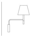
A pivoting metal arm comprising an angled tube that fits into a bracket, also made of metal, hiding the wall plug.
