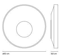
Sun 26 LED 16.2W 700mA 2700K Light source 1890lm Luminaire 949 lm (included)
